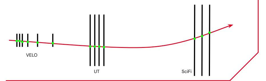
The path of charged particles bends in a magnetic field, just like in the LHC
