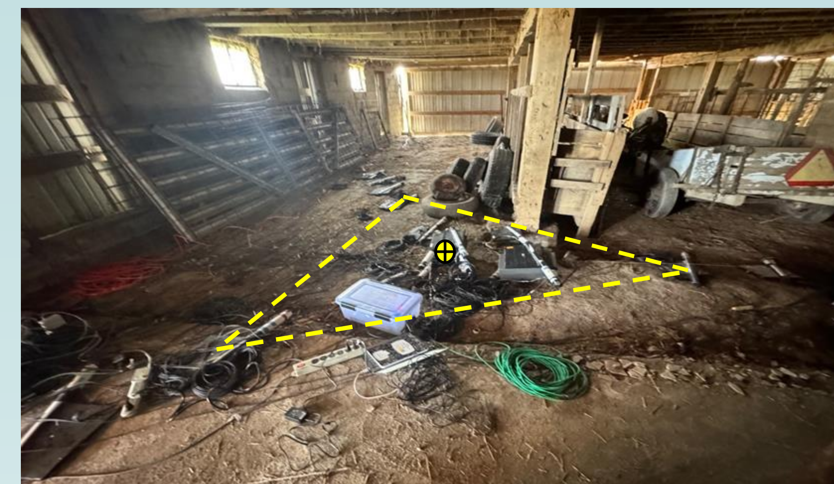
Figure 3. View looking east at the detector array in Westport, IN. The stack of Counter 4 (●) from each detector is at the centroid of the respective triangles. The top vertices are Counter 2 of each detector.
