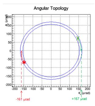
The TOTEM detectors are embedded into the edges of the LHC beam pipe. Each records a "hit" where a scattered proton strikes. The red stars and green Xs represent these hits.
