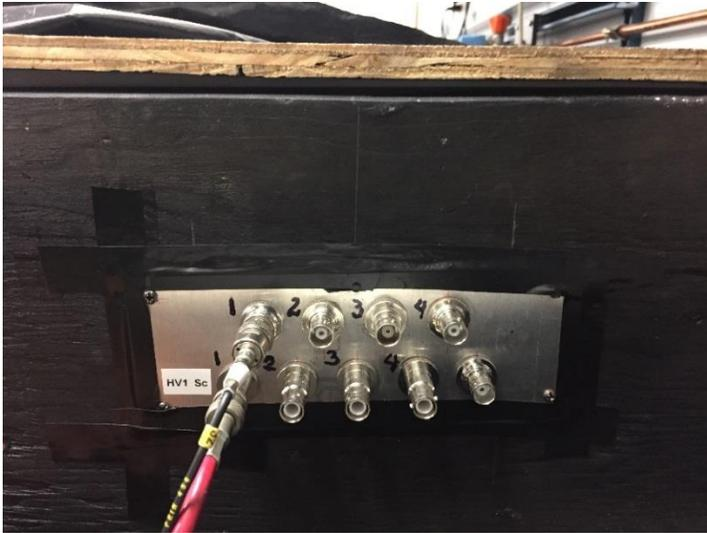
Open connectors and unsealed connector plate.
