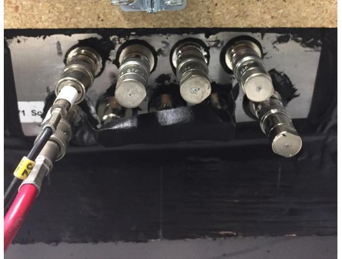
Covered connectors and sealed connector plate.
