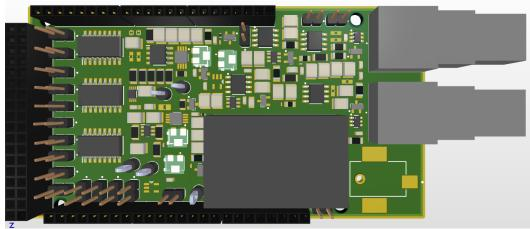
Figure 5: PCB with Arduino Headers
