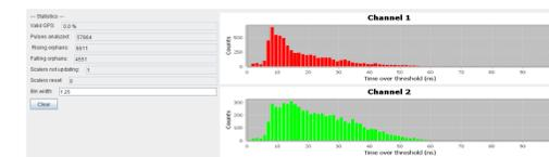
**Fig 11: Time Over Threshold PMT Data**
