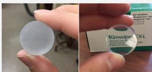
The SCINTILLATOR begins as a square piece of fluorescent acrylic which must be sanded and polished as any imperfections will absorb the light of a muon. Then,
